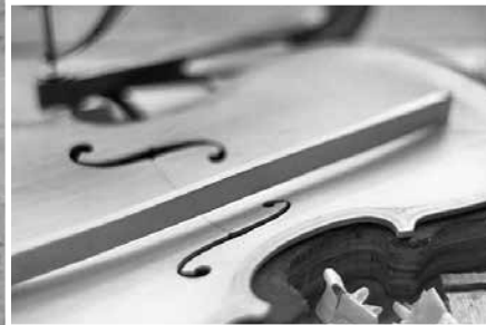
A bass bar ready to be fitted to the top
