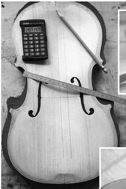
Measuring the top to position the bass bar
