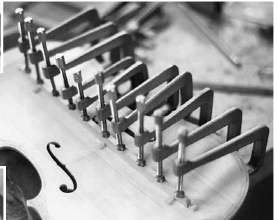
Gluing the fitted bar to the top
